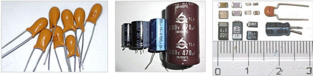
Figure 40: The left picture shows solid electrolyte, resin-dipped 10\ \mu\text{F} 35\text{V} tantalum capacitors (the + sign indicates the positive terminal), the middle image shows 4 electrolytic capacitors of different voltages and capacitance, while the right picture shows miniature low-voltage capacitors above a ruler divided in centimeters.
