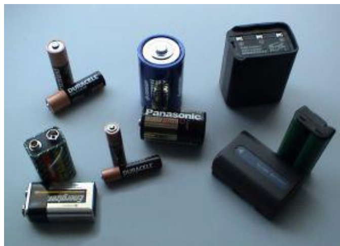
Figure 22: Various cells and batteries (top-left to bottom-right): two AA, one D, one handheld ham radio battery, two 9-volt (PP3), two AAA, one C, one camcorder battery, one cordless phone battery (credit: Wikipedia, http://en.wikipedia.org/wiki/Battery_%28electricity%29 ).
