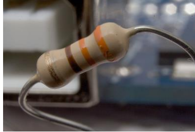
Figure 23: A typical axial-lead resistor. The colors code the value of the electric resistance offered by this resistor (credit: Wikipedia; http://en.wikipedia.org/wiki/Resistor ).
